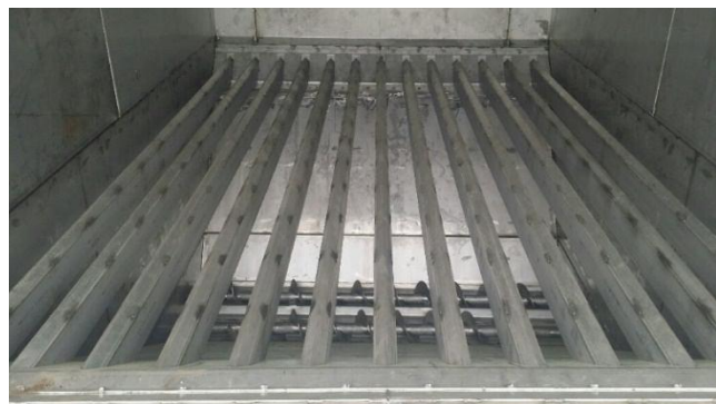
Mixing bunker with 2 screws
